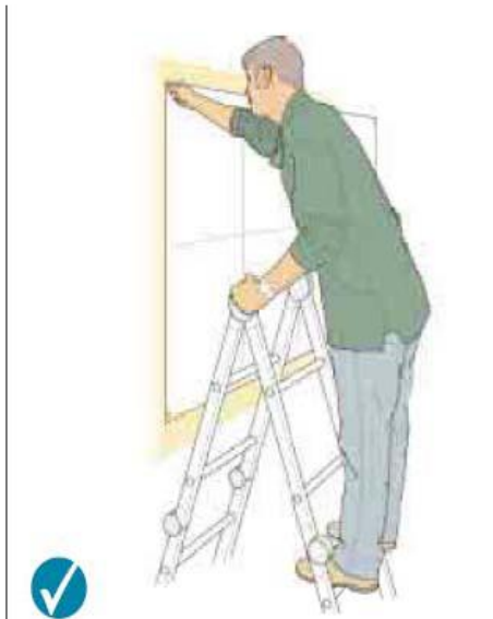
Correct – 2 clear rungs. Don't work any higher on this type of stepladder
